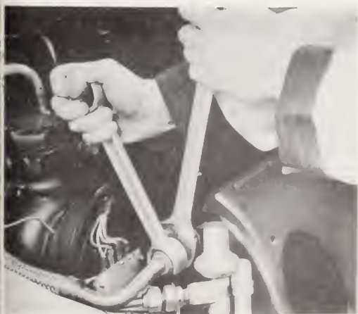
27-27. The correct way to loosen or tighten a flare unit. The flare nut wrench only should be moved. The open end wrench is to keep the adapter fitting from moving or a leak may be started.
